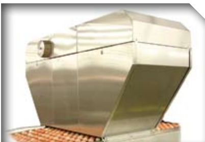
EGGINSPECTOR Able to detect dirty and leaking eggs. Available for OMNIA 125-500
