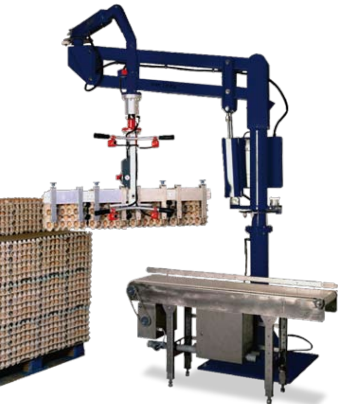
EASYLIFT SYSTEM > Cap. 4 stacks of 6 trays
